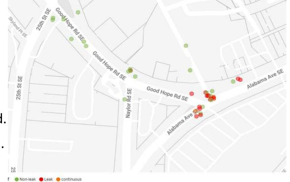
Heat map of the acoustic showing the classification of field result as non-leak, leak, is continuous for the technology.
